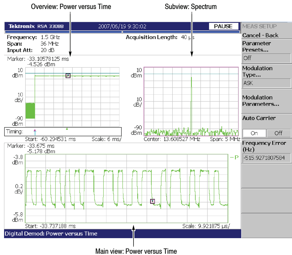
Figure 3-48: Power variance measurement
